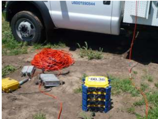
SSC TDMA option on vib' crew using Sigma Acquisition System side by side traditional cable system
