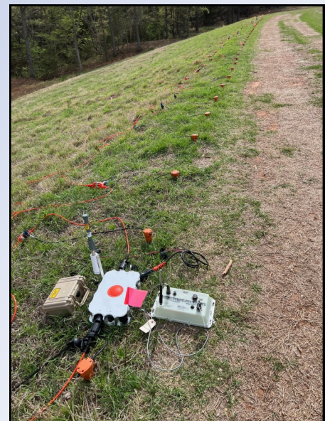
120 Channel U•Node 2 in the field, with attached battery and WTB 4.
