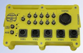
System includes: BD3 11 channel unit (with GPS, Ethernet and Power), Five 4-pin Wireline cables, VibQC Cable Set (with BNC Cables and connectors),
