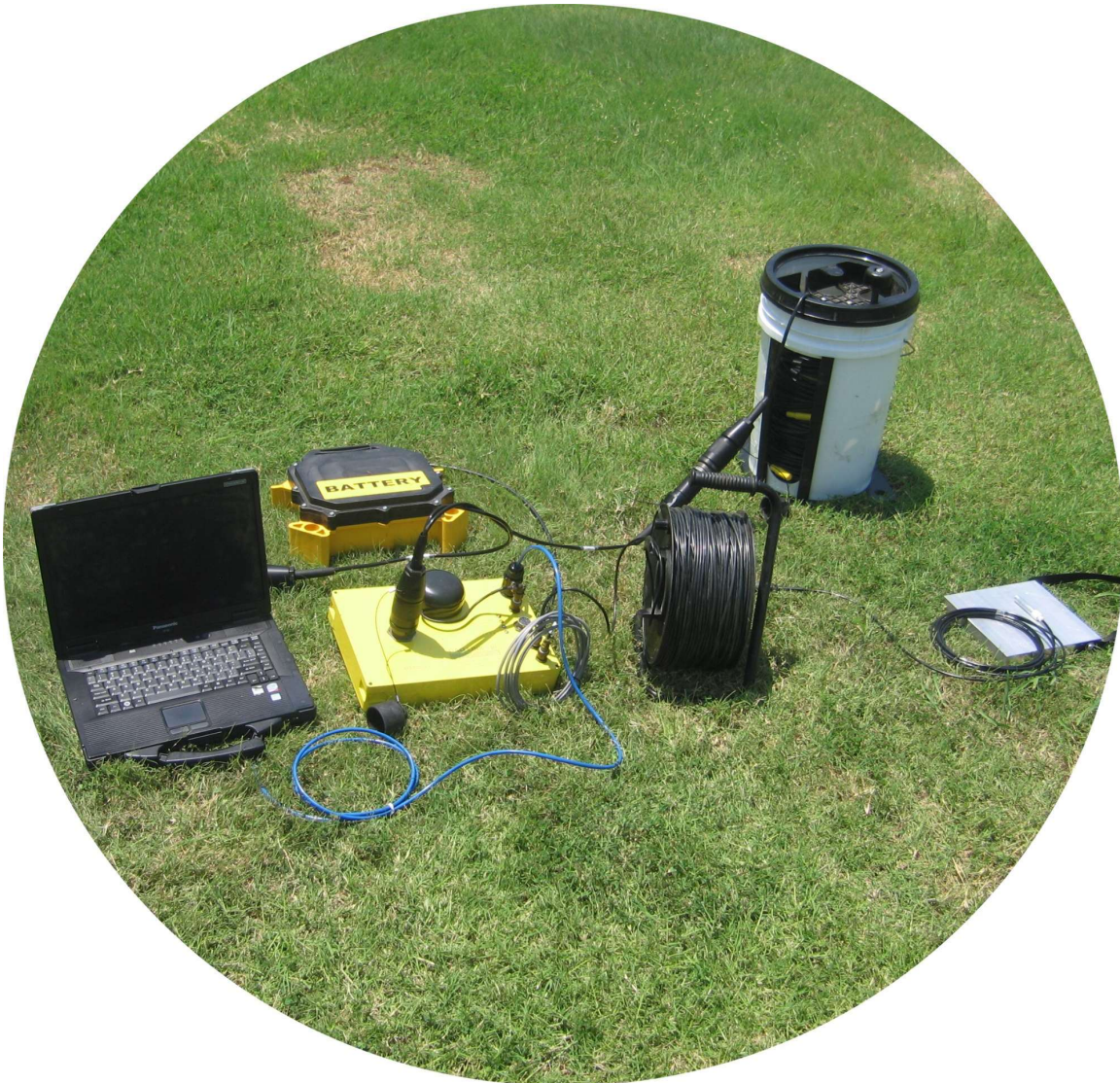
Figure 2.2 – The basic components for a DAQLink 4 System
