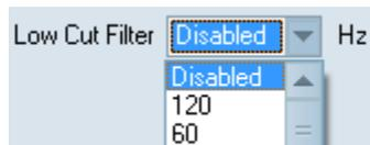
Some plots or test results may be bad if the low-cut hardware filters are enabled. When using a Bird Dog 3-11 unit, the low-cut hardware filters should be disabled. To do this, go to the Options/Preferences menu and select Advanced Mode then go to the Options/Device/DAQ Setup/Configuration window and select Low Cut Filter - Disabled then left click on the OK then Close buttons. After doing that it is almost always best to go to the Options/Preferences menu and deselect the Advanced Mode.
