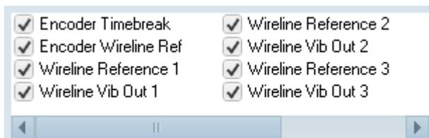
Move the slider below this window to access all the signals that are available. Click on signals to enable or disable them for acquisition.
