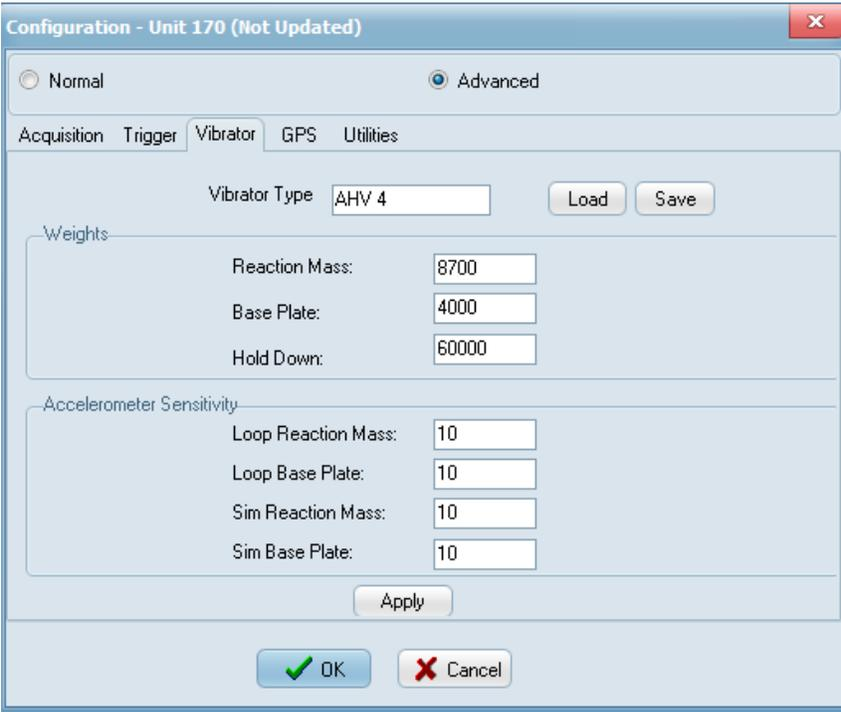
1. Set the Reaction Mass, Baseplate, and Hold Down (Target Force) Weight to match the Vibrator unit that is being tested. All units must be entered in either pounds or Kilograms. All entries must have the same units. i.e. enter everything in pounds or enter everything in KG. Do not enter some items in KG and some in pounds.
