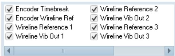
Click to enable or disable signal inputs. Move the slider at the bottom of this window to see all the signals available. This example shows the Wireline Signals List. It is best to only enable active signals for acquisition.
