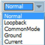
The channel input for each channel may be defined by clicking on the pull-down button for that channel. The only inputs useful for field use are Normal and Current. The other inputs are for testing by Seismic Source personnel. Selecting the Current mode turns on the power supply and current regulator for the channel. Current regulators may be selected for any channel(s) but there are no current regulators (hardware) for channels 9, 10, and 11.
