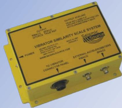
Three main channels: True Reference, Reaction Mass Sim Accelerometer, and Baseplate Sim Accelerometer
