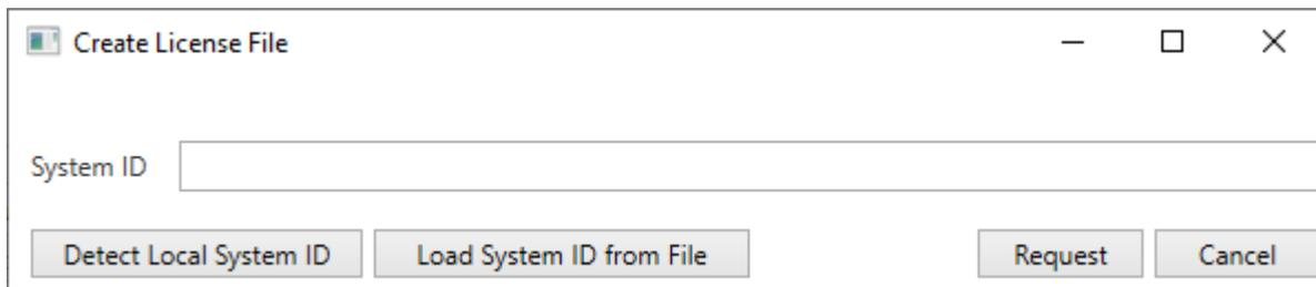
After the System ID is filled in, click on the Request button to initiate the process. Then select the location for the saved license file. The default location is **C:\SSC\Licenses**
