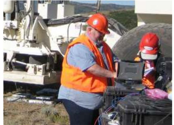
Each Load Cell System uses an Interface Box to gather data from the Load Cells and transmit it to a recording device for interpretation by the provided VScope software
