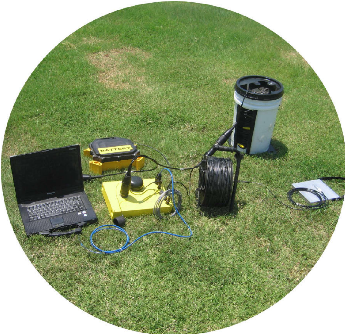
Figure 2.2 – The basic components for a DAQLink 4 System
