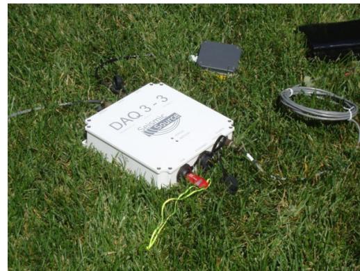
DAQ3-3 with GPS unit and high capacity Lithium battery
